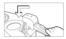
Lower the handle by pulling back the handle release button and lower handle into its recess.
